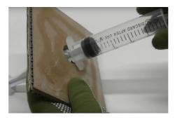
Step 9: Glue the bottle cap to the back of the syringe as shown.
