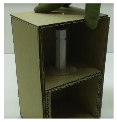
Step 12: Attach the hose to the empty syringe and fill it with colored water. Connect the other end of the hose to the other syringe in our hydraulic press. This way, our hydraulic press is ready.
