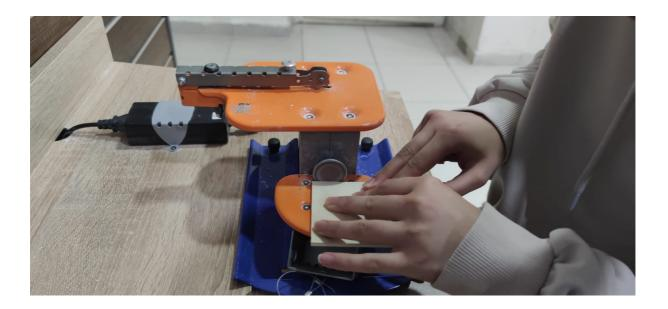
After the filing process, we put dots in the pattern we want on our square plywood. We assign these points to determine where we will drill on the drilling machine.
