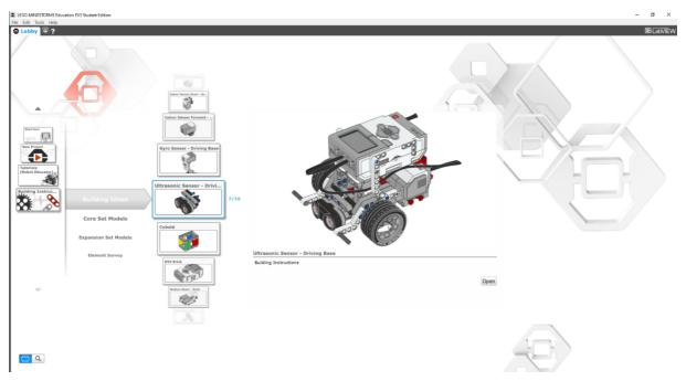
The ultrasonic sensor detects objects and measures distances using high-frequency sound waves. It can detect objects up to a maximum distance of 255 cm.
