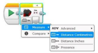
The ultrasonic sensor basically has 2 menus: measure and compare.
